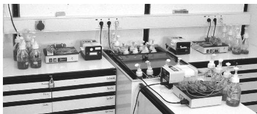
Fig. 5.41: Work place for perfusion cultures is a T-shaped configuration. In the center is a cold box with the storage bottles for the culture medium. Three pumps suck the culture medium from here to the individual work lines.
