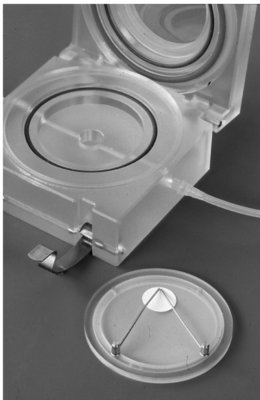
Fig. 5.35: A tissue engineering container used to create tissues with special three-dimensional surfaces under perfusion conditions.
